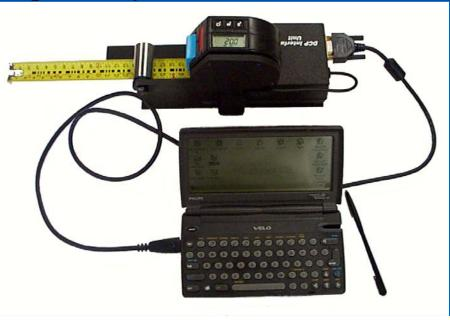
Connect the Tape Measure to the DCP as shown in the figure below.
